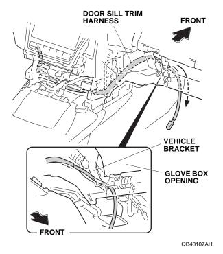
36. Secure the door sill trim harness to the vehicle harness with one wire tie.
