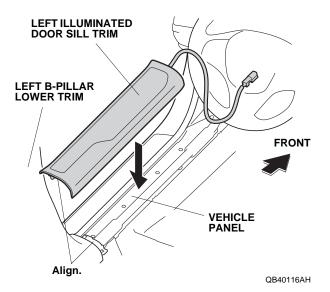
45. Plug the door sill trim harness 2-pin connector into the left illuminated door sill trim harness 2-pin connector.
