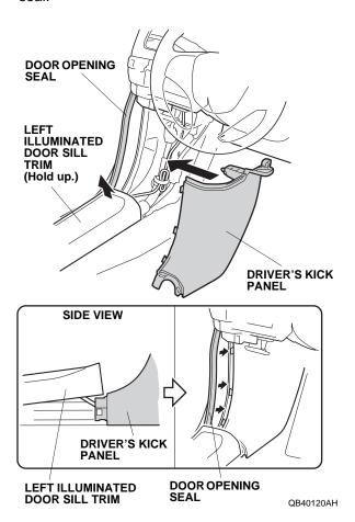
49. Attach the left illuminated door sill trim to the vehicle panel (four clips and six retaining tabs).
