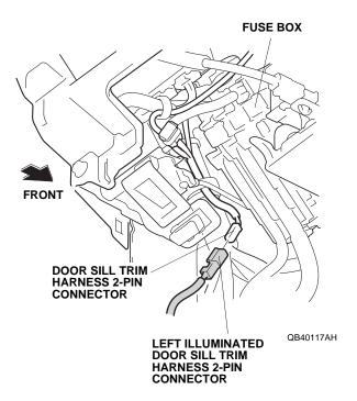
46. Secure the left illuminated door sill trim harness to the vehicle harness with one wire tie.
