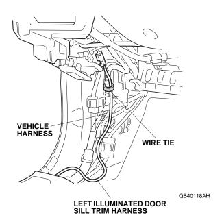
47. Bundle up the excess left illuminated door sill trim harness, and secure it to the vehicle harness with one wire tie.
