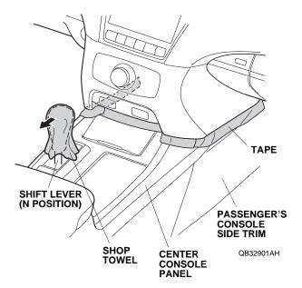
3. Remove the center lower trim (three clips, and unplug the vehicle connectors).
