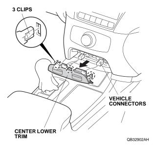
4. Remove the center lower panel (six clips, four hooks, and unplug the vehicle connectors).
