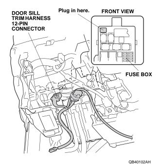
Reinstall the vehicle bracket. Go to step 31. With Another Accessory Harness 12-pin connector
