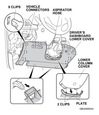
7. Turn the knob, and remove the driver's dashboard under cover (one clip, and unplug the vehicle connector).
