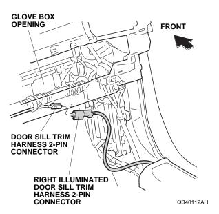
41. Secure the right illuminated door sill trim harness to the vehicle harness with four wire ties.
