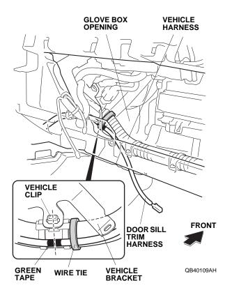
38. Secure the door sill trim harness to the vehicle harness with two wire ties.
