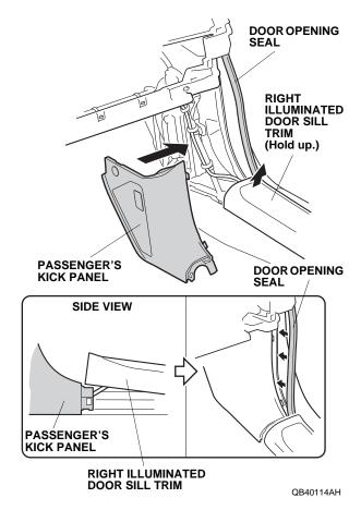
43. Attach the right illuminated door sill trim to the vehicle panel (four clips and six retaining tabs).
