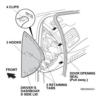
Remove the driver's dashboard lower cover (nine clips, and unplug the vehicle connectors and aspirator hose), then remove the plate (two clips).
