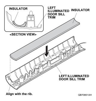
21. Using isopropyl alcohol on a shop towel, thoroughly clean the left illuminated door sill trim where the urethane tape will attach.
