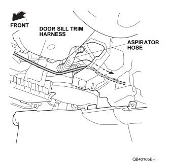
34. Align the green tape on the door sill trim harness with the vehicle clip, and secure the door sill trim harness to the vehicle harness with one wire tie.
