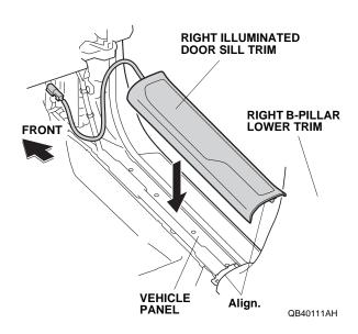
40. Plug the door sill trim harness 2-pin connector into the right illuminated door sill trim harness 2-pin connector.
