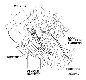
32. Route the door sill trim harness as shown. Align the green tape on the door sill trim harness with the vehicle harness as shown, and secure the door sill trim harness to the vehicle harness with one wire tie.
